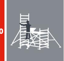
Climb up the built-in ladder, always using the fall arrest safety harness with a shock energy absorber and an anchorage point. Insert the two upper lateral frames by inserting them into the tenons of the lower lateral frames. Introduce the metallic interlock clips also into the lower hole (in order to join both lateral frames). After that, assemble the corresponding horizontal and diagonal braces.
